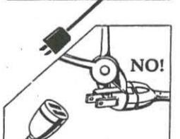
Don't do it! The third prong is there because the appliance must be grounded to avoid electric shock.
